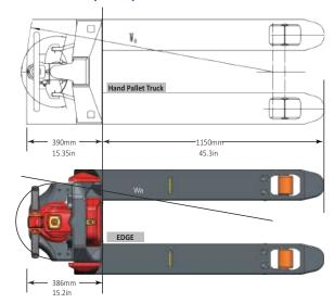
The short body length of truck (L2=380mm) is even smaller than Hand Pallet Truck. it provides the shortest turning radius of 1274 / 1336 mm with lifted/lowered forks and makes the truck extremely compact and ideal for use in confined spaces of retail stores, elevators or business centers.
