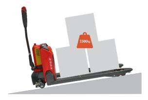
Load capacity of 1500 kgs, rugged drive unit and high gradeability make the truck an ideal choice for rigorous short distance transfer duties, clearing of staging areas and operating on ramps.
