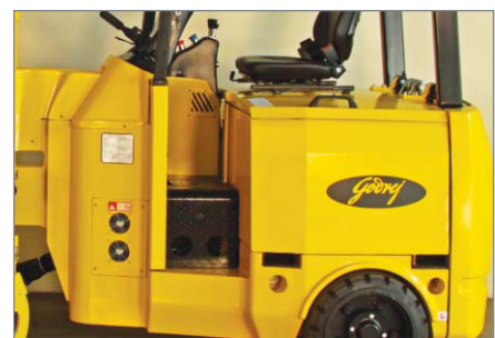
Single allen key required to access control units
