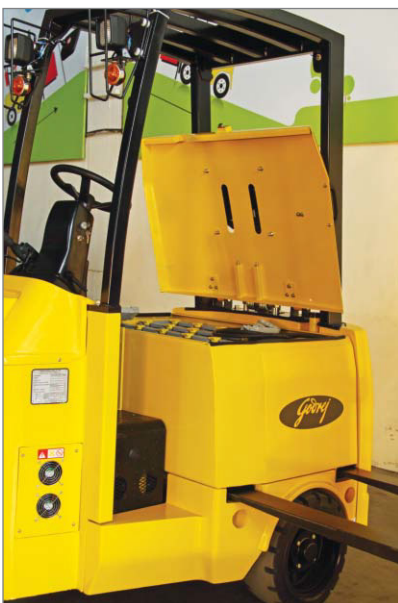
Fork pockets for easy removal of battery
