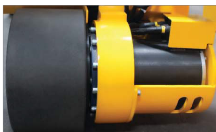
Easy access to AC drive motors
